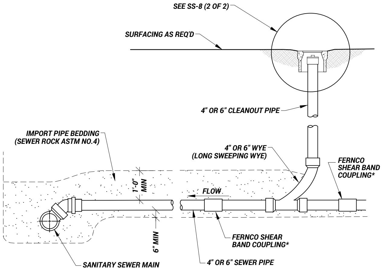
\*NOTE: FERNCO SHEAR BAND COUPLINGS USED FOR LATERAL REPAIRS ONLY.
