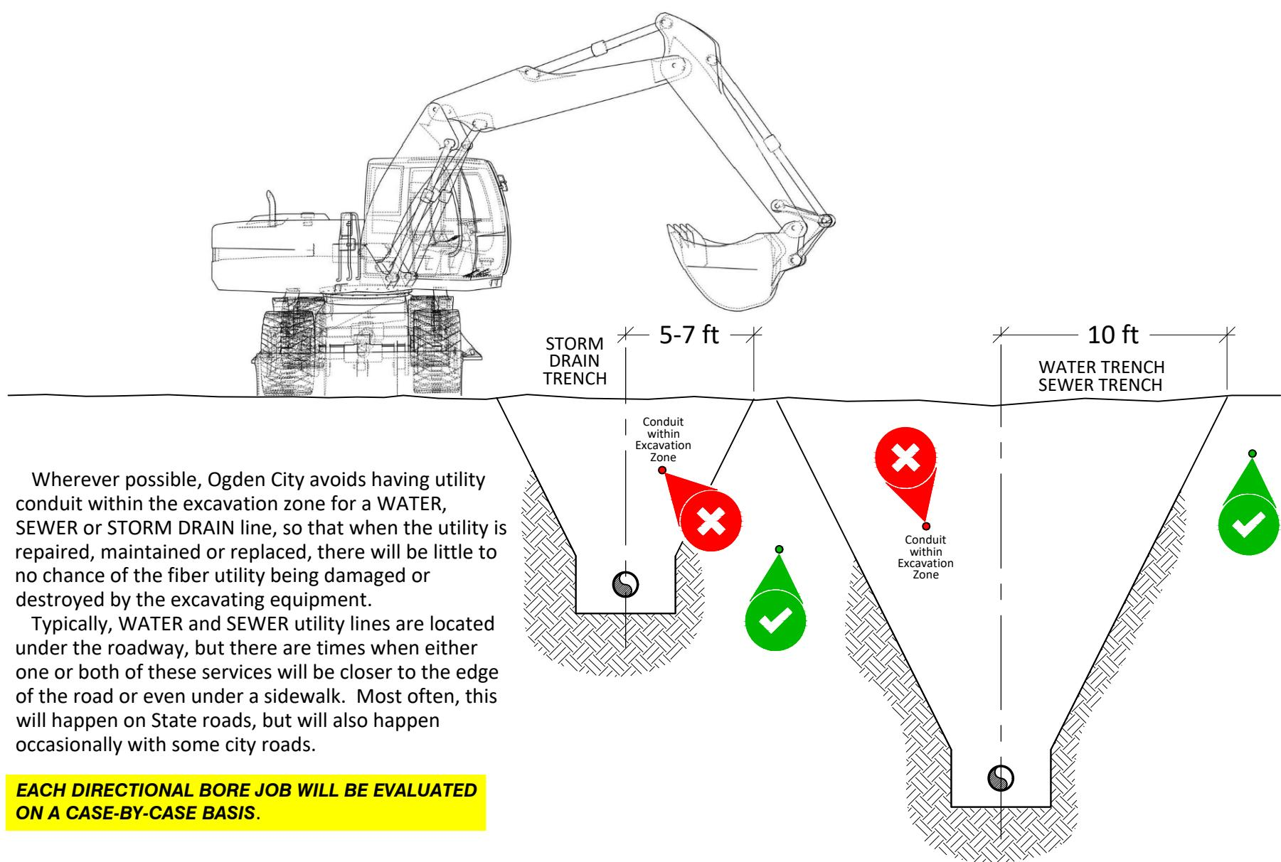
Wherever possible, Ogden City avoids having utility conduit within the excavation zone for a WATER, SEWER or STORM DRAIN line, so that when the utility is repaired, maintained or replaced, there will be little to no chance of the fiber utility being damaged or destroyed by the excavating equipment.
